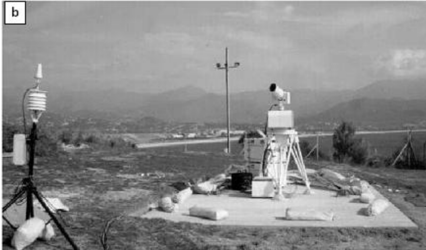
Figure 3: French Transportable Laser Ranging Station. (a) Main components of FTLRS (b) Photo of FTLRS during the Corsica campaign (on left, one can distinguish the meteorological station and GPS antenna).
