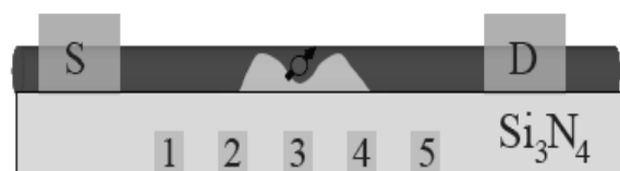
Figure 01: Real model of the single electron transistor [11]
